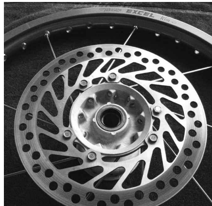
Left: The new pieces, left, are visibly more substantial than the stockers they replace. (Don't be fooled by the narrower threaded section on the Excel spoke; its shaft is thicker than OEM.) Right: The first row of new spokes, with nipples loosely attached. Right: Notice the even spacing along the rim.
