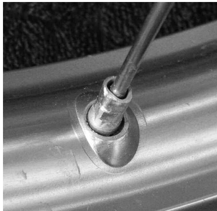
Left: A perfect fit between spoke wrench and nipple makes the job easy and... (Center) prevents this from happening. Not only is this nipple rounded, it's also become crushed against the spoke threads, making it doubly difficult to remove. Right: Once loosened "topside" with a wrench, nipples can be unscrewed easily from the other side.
