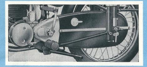
Lifetime of the driving chain is considerably prolonged by the dustproof chain guard. Small lids on it facilitate the maintenance of the chain and the dismounting of the rear wheel
